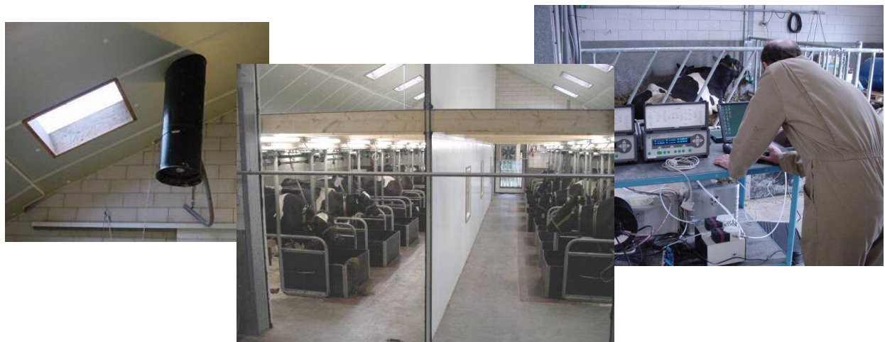
Figure 4.2: The two equal halves of the experimental barn at De Viersprong with equipment to measure methane.
